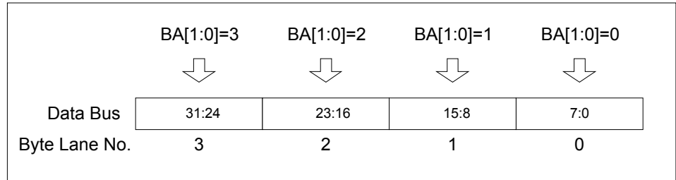
Figure 3-2. Little-Endian Mode Addressing
